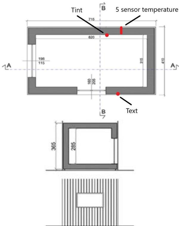
Fig. 2. Planimetry, vertical section B-B and the prospectus with the window of the straw house.
