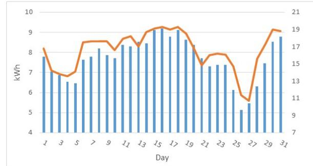
Fig. 9. Daily energy consumption of the electric heater in December 2016 with the temperature differences between inside and outside environments (in orange, °C).
