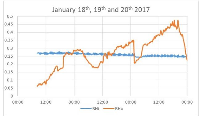
Fig. 7. Experimental campaign in January 2017: measured relative humidity in the inside (i) and outside (o) environments.
