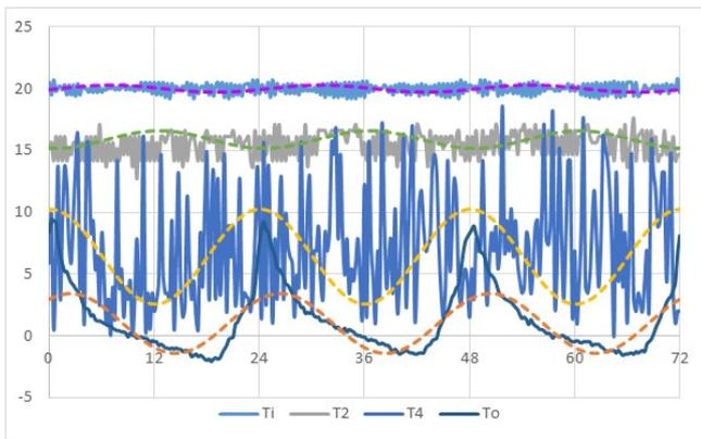
Fig. 6. Experimental campaign in February 2017: measured temperatures inside the straw wall (T1-T5) and calculated sinusoidal variations of temperatures with the dot lines (°C).
