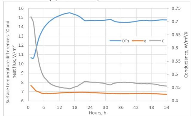
Fig. 4. Average method results of surfaces temperature difference  $DT$  ( $^{\circ}C$ ), specific heat flux  $q$  ( $W/m^2$ ) and conductance  $C$  ( $W/m^2/K$ ).
