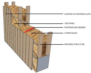
Fig. 3. Wooden straw structure of walls and temperature sensors.
