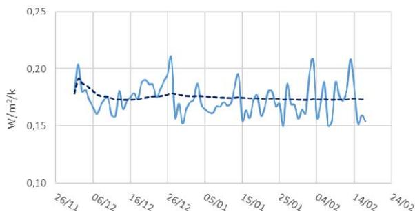
Fig. 10. Simplified method to evaluate the average thermal transmittance of the building envelope by the energy consumption of the electric heater.
