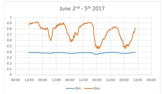
Fig. 8. Experimental campaign in June 2017: measured relative humidity in the inside (i) and outside (o) environments.
