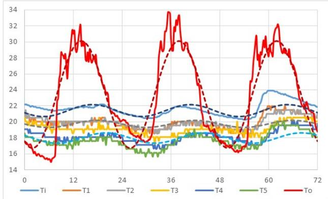
Fig. 5. Experimental campaign in May 2016: measured temperatures inside the straw wall (T1-T5) and calculated sinusoidal variations of temperatures with the dot lines (°C).
